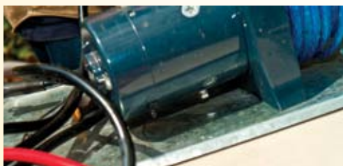
While it was clear the motor enjoyed its bath in the river, the drain holes did their bit releasing water the whole time during removal of the winch
