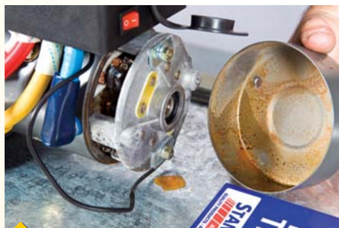
The motor had signs that water had made an appearance, with corrosion already starting to form on the internals and droplets still lingering around the vital components. But we guess if you consider the manufacturer states clearly that this winch is not to be used in water or mud, it did reasonably well outside of its comfort zone
