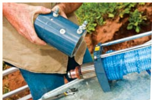
The gearbox itself remained fairly dry, allowing the grease to stay clean and protect the gears. It only showed the slightest sign of water that dribbled out from the drum area once the gearbox was removed
