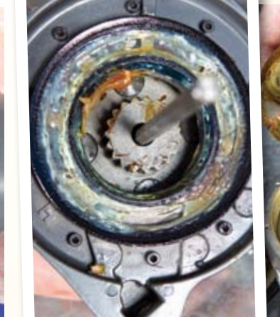
The gearbox was sealed up surprisingly well for a budget winch that's not recommended for mud and water. There were small droplets that had made their way into the top section of the planetary gear set
