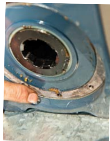
The gearbox itself remained fairly dry, allowing the grease to stay clean and protect the gears. It only showed the slightest sign of water that dribbled out from the drum area once the gearbox was removed
