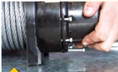
The gearbox had gaskets in all the critical mounting locations, but unfortunately it didn't hold out water during our test. As we split the gearbox, it let out a dribble of water and droplets were found around the gears as well
