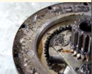
The gearbox had gaskets in all the critical mounting locations, but unfortunately it didn't hold out water during our test. As we split the gearbox, it let out a dribble of water and droplets were found around the gears as well
