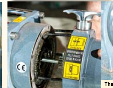
The gearbox was sealed up surprisingly well for a budget winch that's not recommended for mud and water. There were small droplets that had made their way into the top section of the planetary gear set
